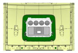
5. Installation of pull - lined pressure plate (Torque :15NM)
